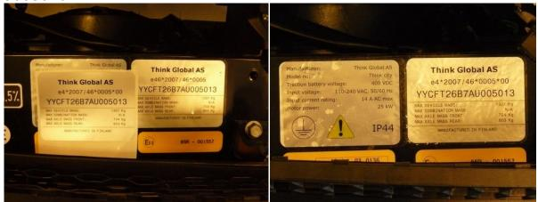
Remove the old type approval mark to replace it with the correct label. Attach the foil over the label.
