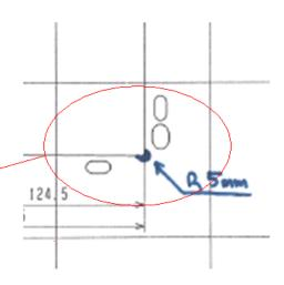
All 4 corners to be grinded as showed on pictures below. (Mickey Mouse ear) Be sure to have a smooth surface and no sharp edges when finished (Grind with a fine grade)
