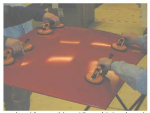
Apply BetaSeal 2700 to primed area. Adhesive string 10mm wide x 15mm high, placed 5mm from outer edge of primer. Turn roof right way up. Fit 4 location fixtures along cantrail. Center quarterlight and center door. Fit Roof to location fixtures and remove vacuum grippers.
