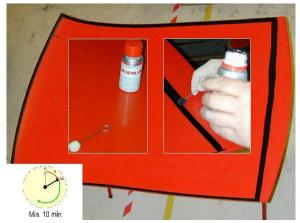
Apply BetaClean 3350 on inside along front and side edges, minimum 25mm stripe, and at the rear. Wipe on and wipe off in one direction only, using lint-free paper. Let cleaner dry. Shake Primer 5404 box for min.1 minute after loose ball. If container is not opened for the first time, make sure primer is no more than 5 days old.
