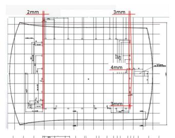
Grind of plastic panel in front & rear according to mark-up below. Be sure to have a smooth surface and no sharp edges when finished (Grind with a fine grade)
