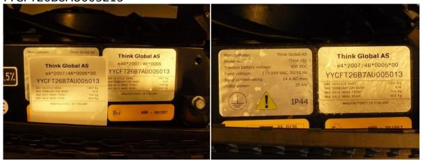
Remove the old type approval mark to replace it with the correct label. Attach the foil over the label.
