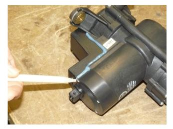
Apply glue all around the cover at the edge of the pump.
