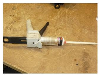
Use 3M DP 410 glue, a glue gun and a mixing tip as this will provide the right mix of glue and hardener
