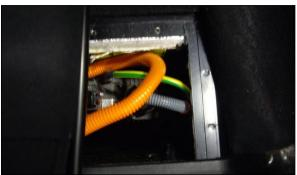
Locate the AC-heater connector, and carefully unplug this.
