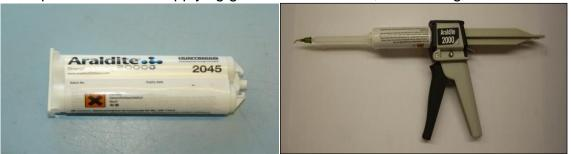
3: Insert sealant applicator needle through the hole in the tube, and insert Araldite 2045 while rotating the tip gently in a circular motion, trying to apply sealant in all directions to create a complete seal. Keep applying pressure while removing the needle from the tube, to also fill the hole created in the tube.
