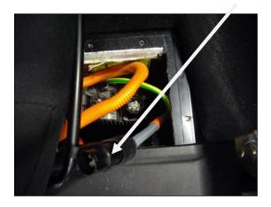
Using dry compressed air and a nozzle gun, dry out possible humidity in the connector by pressing the nozzle gun into each unpopulated terminal position and releasing air for approx. 20 seconds.
