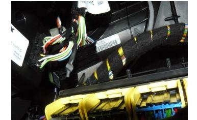
Isolate the cable by using shrink tube and hot air gun. Confirm that it is not possible to ground the wire.
