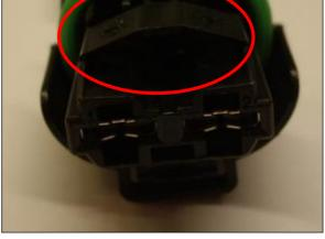
2. Carefully, using a terminal release tool, release locking tabs inside the connector-housing, and pull terminal 1 and 2 free from the connector-housing. Scrap the connector housin
