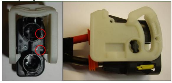
7. Press secondary locks firmly into locking position
