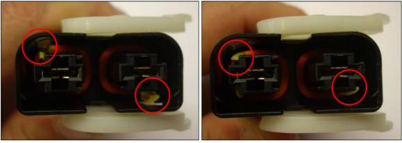
8. Test, using only gentle hand force, by pulling, if cables are properly located and locked Mark cable label with text: "GEN2 adaptation"
