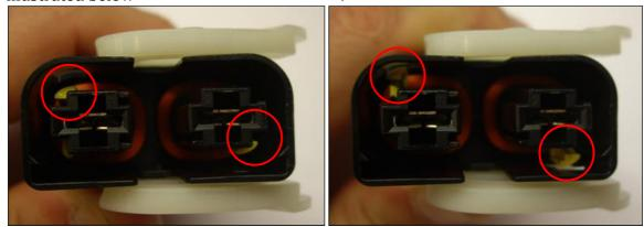
5. Release cables from connector, and scrap GEN2 harness. Keep only the connector
