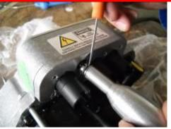
To remove the interlook with an enab tool and a screwdriver
