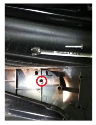
Next, place a M6 long extruded U-nut, (S&S part #J5650PK) in the center of the existing hole.
