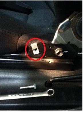
Insert M6x40 bolt (S&S part#J65337) through hole and into threaded U-nut and tighten snugly.
