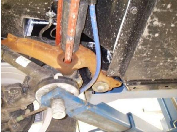
**Rear lifting point when replacing the battery:** On the damper fastening on the control arm ensuring enough space for the battery tray when the tray is lowered. The same on the opposite side.
