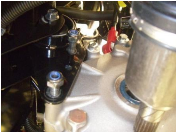
Rear motor bracket (on the gearbox)
