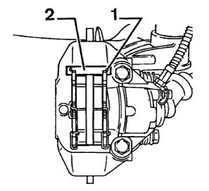
Press the stop plate in (2) after applying a **thin** layer of copper paste on both sides. Install new cotter pin (1). Fit the wheels.
