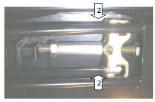
Verify that both seconday cables (2) connected to the compensator move in parallel.
