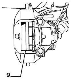
Apply a **thin** layer of copper pasta on the lower glide track for the brake pads (9).
