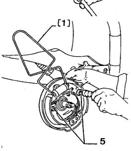
Install the clamp [1] on the brake cylinder.
