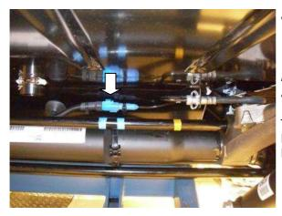
Disconnect the blue connector and unhook the cable from the fastener.
