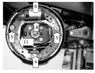
Install the handbrake cable behind the bracket (11).
