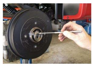
Remove the washer (for example with a magnetic tool) before pulling the drum off.
