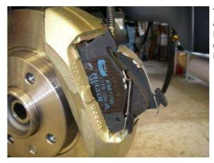
Tilt the upper edge of the outer brake pad out and remove it.
