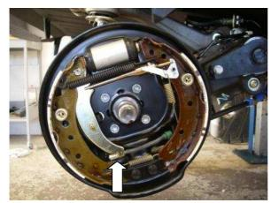
Before assembling the brake shoes the handbrake cable must be connected to the arm.
