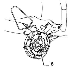
Pull the brake shoes apart and loosen them from the lower fixing points.
