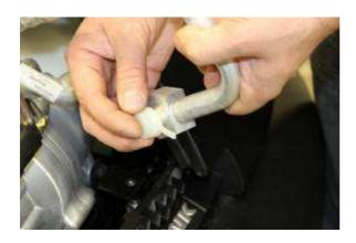
Important: Install plugs in, or tape over the opened refrigerant line fittings and compressor ports.
