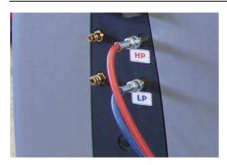
Use an AC service unit with two connections, for HP and LP (high pressure/low pressure)
