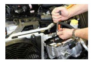
Disconnect the A/C discharge line from the condenser.
