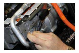
Disconnect the supply connector from the A/C compressor.
