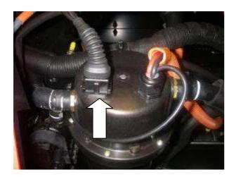
Disconnect the connector on the fluid heater.
