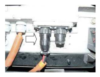
• Disconnect the connector to the fluid heater.
