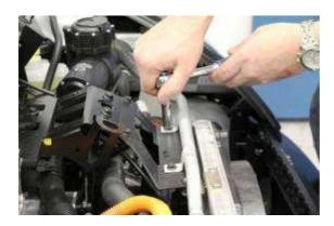
Remove the 4 attaching bolts on the mounting bracket
