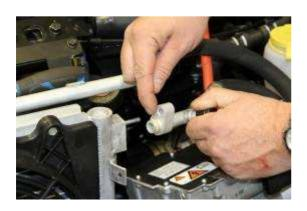
Replace rubber O-ring. Lubricate the rubber O-ring with clean refrigerant oil before installation.
