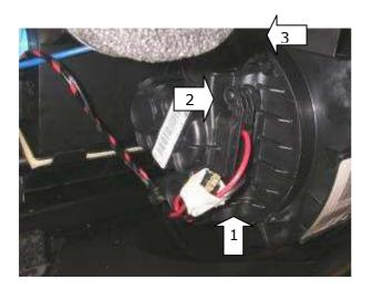
It is now possible to access the blower and loosen it. It is also probably possible to wriggle the blower down between the steering column and the heater. To do this the heater must be moved slightly to the right. If this is not possible the complete dashboard must be removed before the blower is removed.
