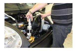
Carefully lift condenser up, and remove it from the engine compartment.
