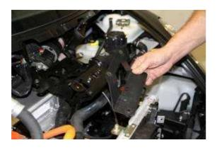
Release the condenser support bracket.
