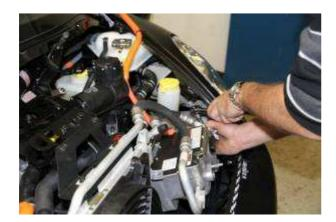
Disassemble the compressor support bolts.
