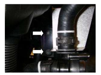
Loosen the fluid heater bracket and remove it.
