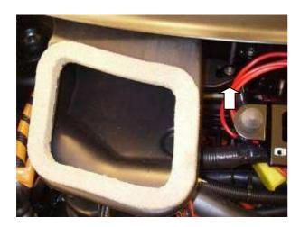
Remove the air duct above the fluid heater for easier access to the fluid heater and the coolant hoses. The air duct is fastened with one fastener.
