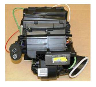
Note: AC equipped Evaporator cannot be serviced separately. The complete unit must be replaced
