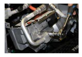
Remove the nut that secures the A/C discharge line to the compressor
