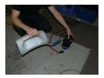
**TIP:** When replacing the fluid heater it is necessary to fill the new fluid heater with coolant before installing it. This will make the bleeding process easier and faster.
