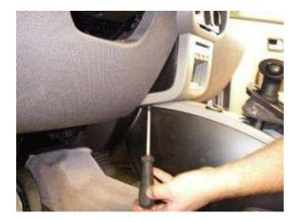
Loosen two fasteners at the bottom; one on each side of the center stack (one side shown in the picture).
