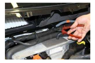
The front "H" valve-type thermal expansion valve
