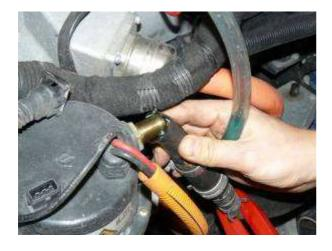
When the pump is running smoothly and all air is out of the system the bleeding tool can be disconnected in followed steps:
