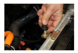
Take care of rubber bushing when the support bracket is removed.
