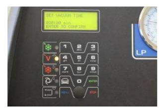
Start the evacuating of the system. For correct "vacuum" time se technical data.
