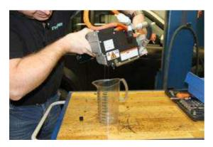
Drain the compressor for refrigerant oil and measure the amount of oil. Add the same amount of oil into the refrigerant system, when installing the new compressor.
