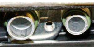
Inspect rubber O-rings and tube flange for damage.
