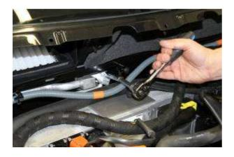
Remove the bolt securing the refrigerant lines to the expansion valve (TXV).
