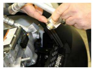
Inspect seals and tubes for damage.
