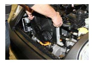
Carefully lift the condenser up and hold it.
