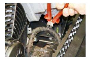
Remove cable ties from the wiring harness.
