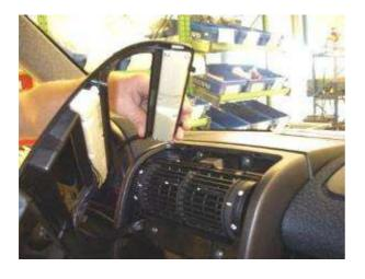
Remove the frame with indicator lights. The frame is fastened with clips.
