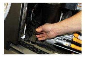
NOTE: Inspect that the rubber bushings located under the condenser are in correct location after removal.
