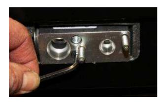
Remove the bolt securing the expansion valve to the evaporator
