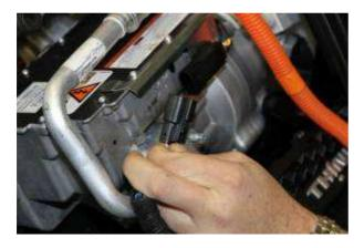
Disconnect the wiring harness connector at compressor.
