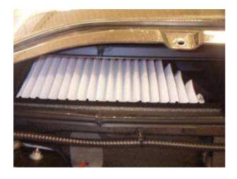
Remove the old Fresh air filter and install a new one.
