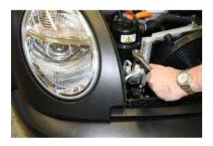
Disconnect the discharge line from the receiver/drier.
