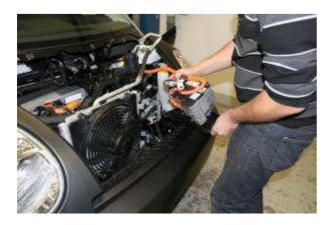
Carefully lift the compressor up, and remove it from the engine compartment.
