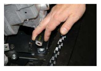
Disassemble the ground cable.
