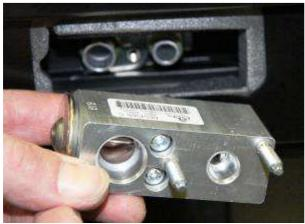
Carefully remove the expansion valve from the evaporator.
