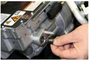
If refrigerant oil has been drained from the A/C compressor, the same amount of oil should be added to the refrigerant system. (See specifications for correct oil type.)
