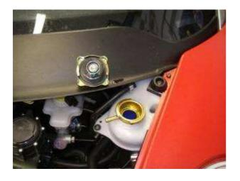
• Fill coolant to the MAX level on the reservoir and leave the cap off.
