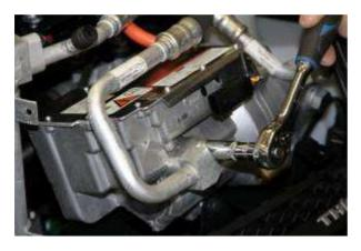
Remove the nut securing the suction line fitting to the top of the compressor. Disconnect the suction line fitting from the compressor suction port. Remove the seal from the suction line fitting
