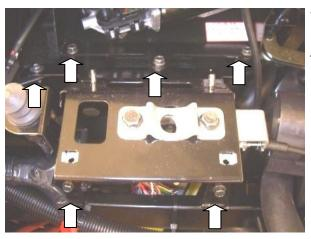
To access the wiper motor you first have to loosen the hood latch bracket with the junction box.
