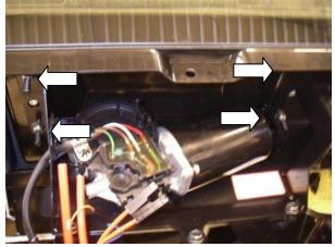
Loosen the four fasteners for the wiper motor bracket. The wiper motor can then be removed complete with bracket.
