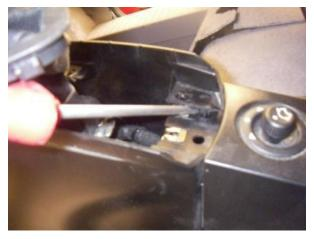
Loosen fastener and tilt the back of the panel releasing the plug and pull the closure panel off.
