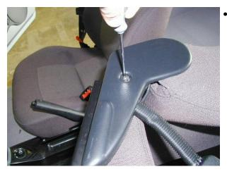
Loosen belt tensioner/belt fastener cover.
