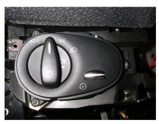
The main light switch has 3 fasteners.
