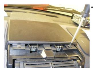
Loosen the center stack top plate.
