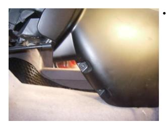
Loosen the two gear console closure panel fasteners.
