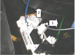
The picture is showing the wire for heating and ventilation connected to the back of the control panel. Electrical contact is here already disconnected.
