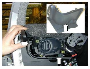
Remove the frame arount the instrument panel and main light switch.
