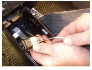
Disconnect the electrical window switches.
