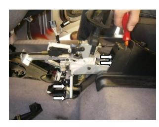
Bracket with gearshift can now be disassembled.
