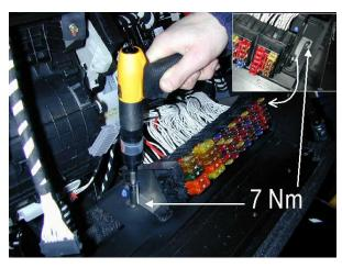
• Loosen the two fusebox fasteners.
