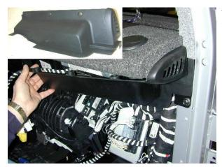
The passenger's side panel has five fasteners.
