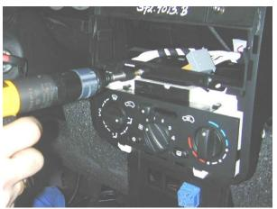
The control panel with buttons for heating and ventilation can either be taken out individually or together with the frame.
