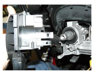
Loosen clips on boths sides of the steering column and pull the clock spring out.
