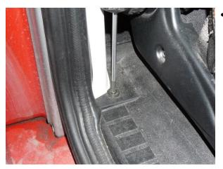
Loosen the fastener and remove the panel.
