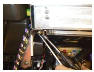
The airbag itself is fastened to a separate frame with four nuts.
