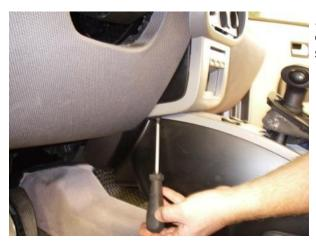
... and two fasteners at the bottom; one on each side of the centre stack (one side shown in the picture).
