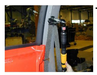
Loosen the upper seat belt fastener.
