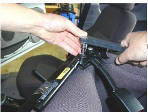
Loosen belt tensioner and belt fastener.
