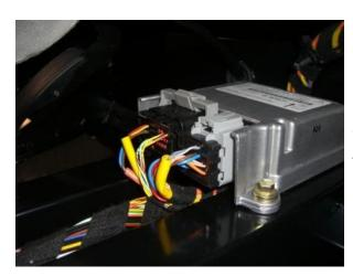
Disconnect cables and unfasten the control unit.
