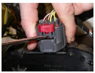
To release the accelerator pedal contact the red locking mechanism must be pressed upwards and the barbs pressed in (see picture).
