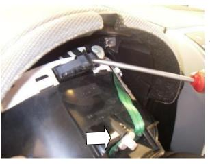
Tilt the instrument panel contact locking mechanism and pull it loose.
