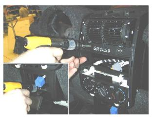
The inner frame around the control panel and center vents can now be disassembled. It has 4 fasteners. The frame can now be removed together with center vents, control panel and switches/connections on the back side.
