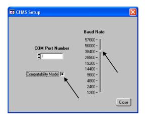
Check"Compatability Mode" and select "Baud Rate 38400".
